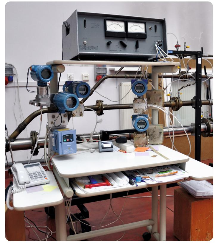
Workstation for testing flow in ventilation installations.
