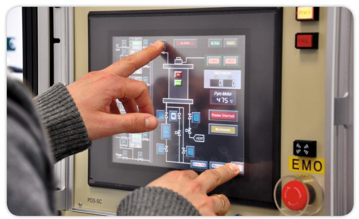
Control panel for the technological plasma system for synthesis of diamond layers.
