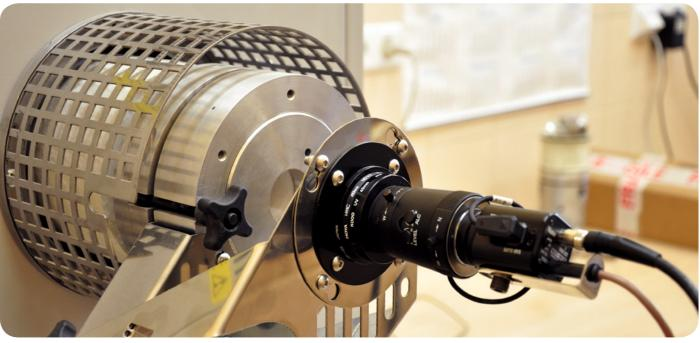
Analyzer for characteristic ash fusibility temperatures.
