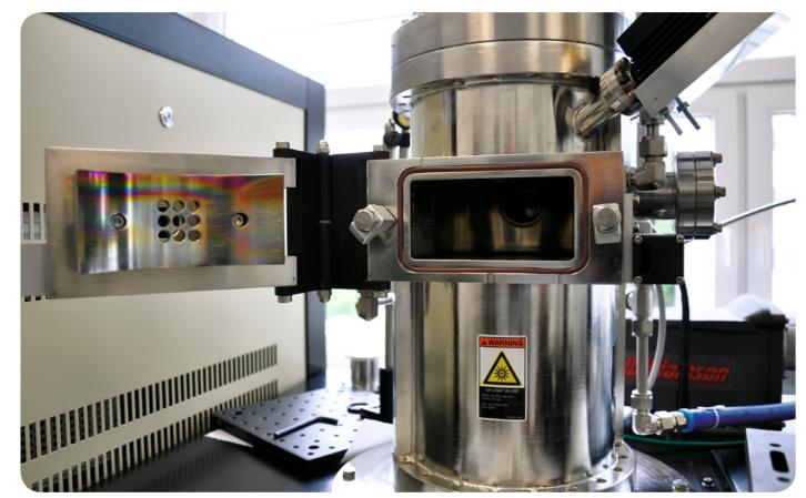
Plasma vacuum chamber for synthesis of diamond layers.
