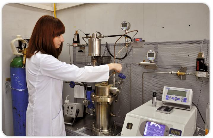
Laboratory installation for coal gasification and pyrolysis.
