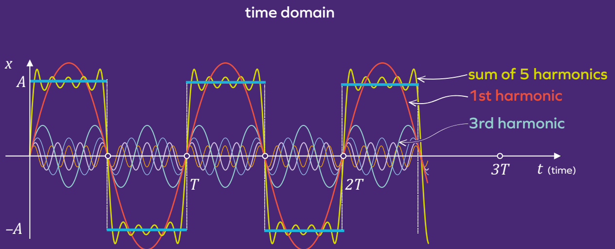
Fig. 8. Harmonics of the square wave in time domain.
