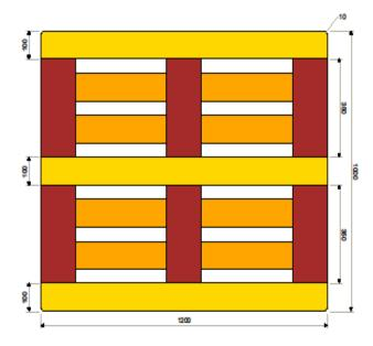
Nails/Joint: Deck board/Block 2 pcs. 3.1/85 mm ring nail
