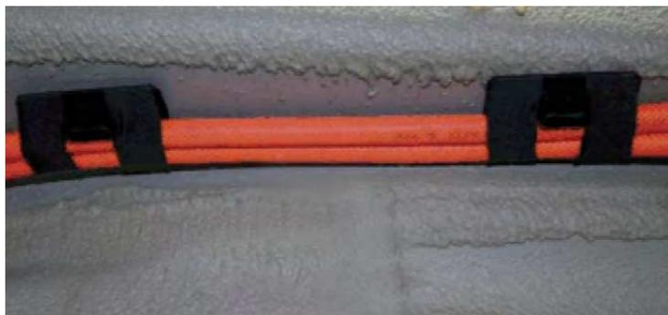
High-voltage cables can be identified by the orange-coloured insulation or coating.
