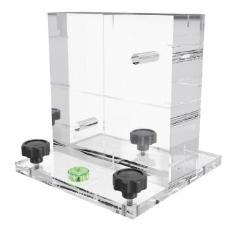
This phantom can be used to check the alignment of the internal and external lasers to the radiographic center of CT and PET/CT units and to verify lateral gantry angle. It can also be used with accelerator units to check vertical and lateral gantry angles, laser alignment and vertical table movement.
