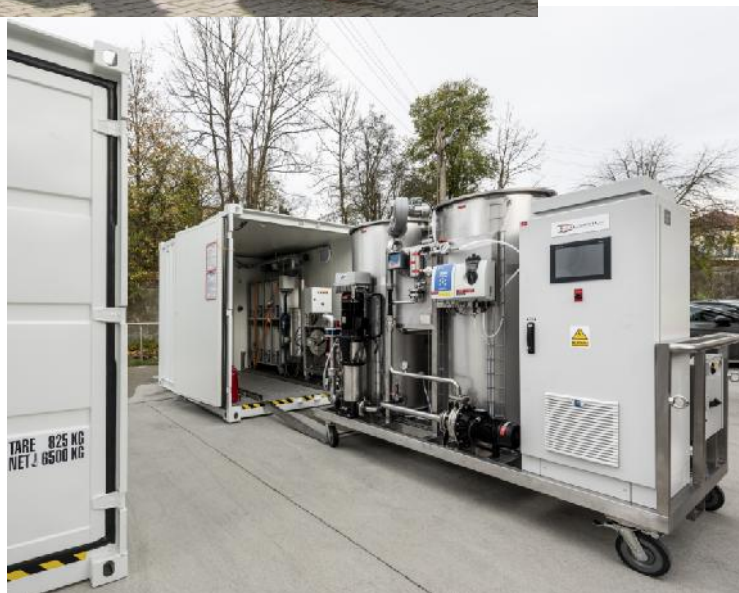
SPID for production of degassed highly-ozonated water 20 m 3 /h
