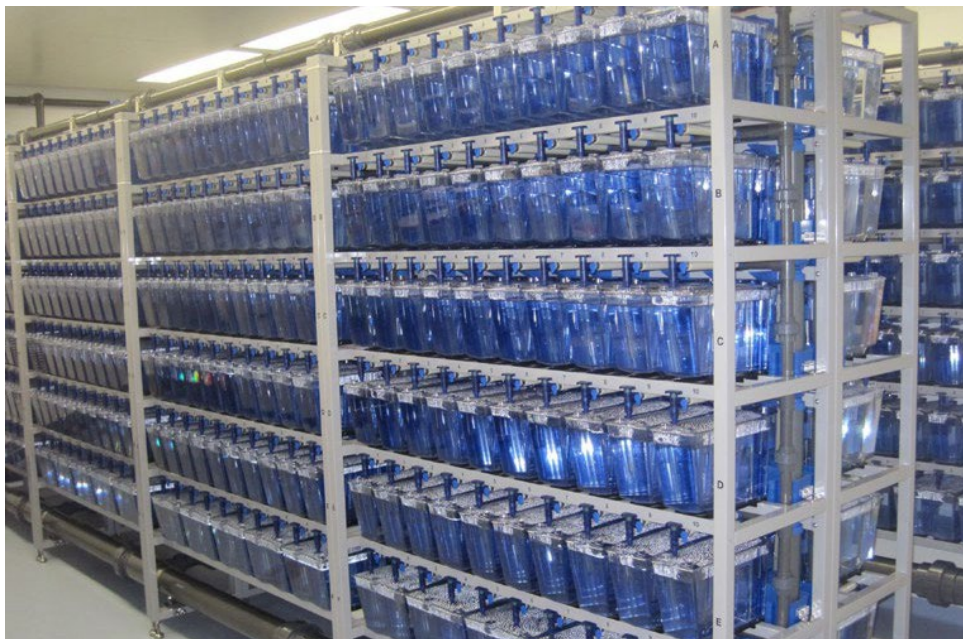
Figure 5.11. Multi-rack system showing several connected racks for Zebrafish
