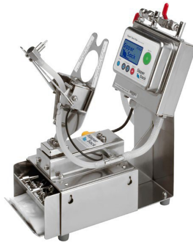
Figure 7.13. Apparatus for filling and sealing water bags
