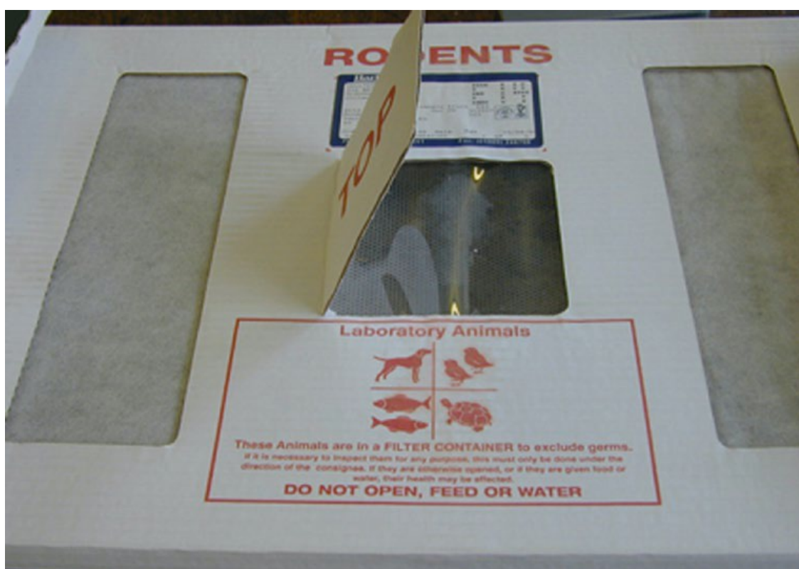
Figure 11.1. Transport box for small laboratory animals showing viewing window
