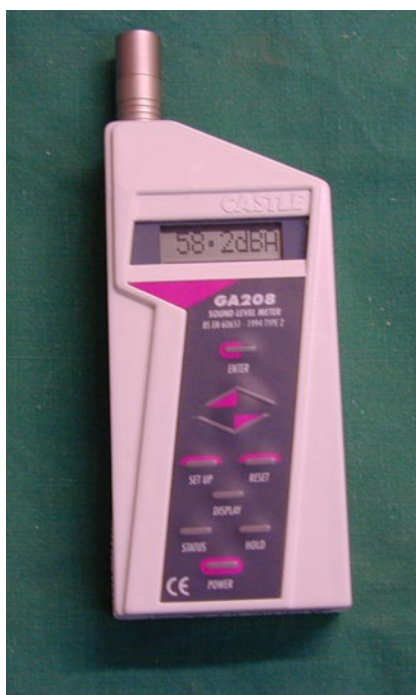
Figure 5.20. Sound meter reading 58.2 dBA
