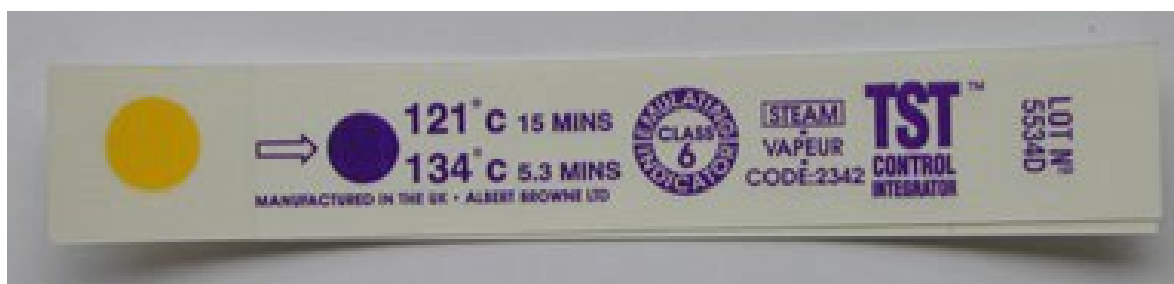
Figure 6.25. Indicator strip. The yellow dot changes to blue after the temperature has been reached for the required amount of time
