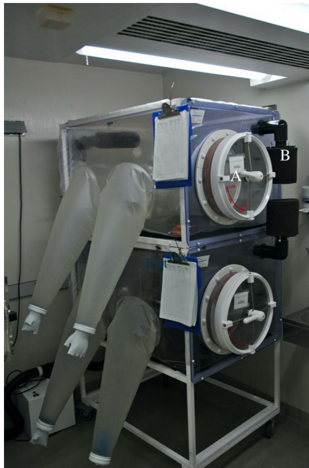
Figure 4.3. Flexible film isolators. A = entry port; B = Filter for air extract
