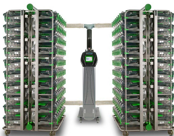
Figure 5.7. Racks of IVCs
