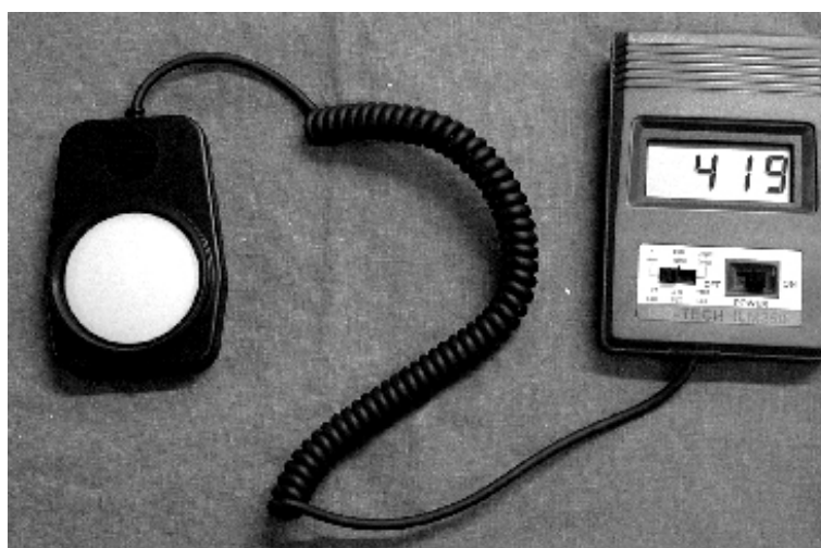
Figure 5.18. Light meter reading 419 lux
