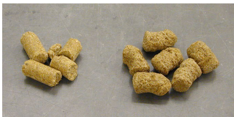
Figure 7.2. Compression pellets (left) and expanded pellets (right)
