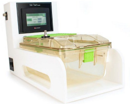
Figure 12.3. A carbon dioxide euthanasia system designed to hold a specific cage
