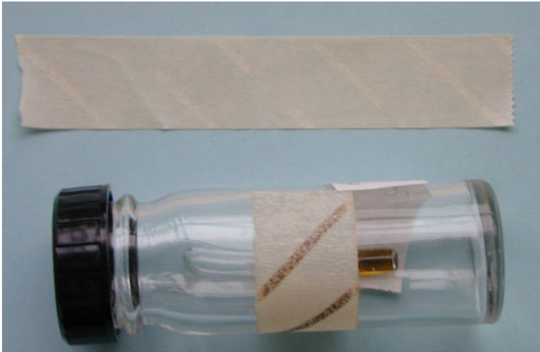
Figure 6.24. Autoclave indicator tape. Top: appearance before autoclaving. Bottom: appearance after autoclaving
