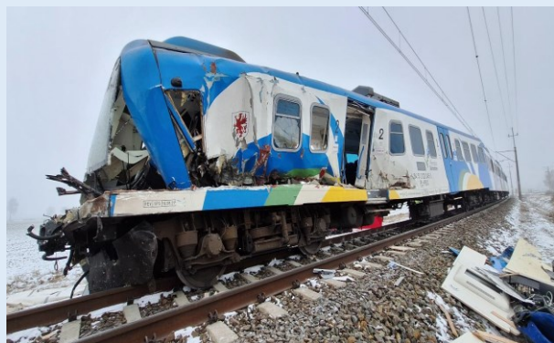
Photograph 1 - Consequences of the occurrence - the damaged EMU EN57AL-1527 (source: own material of PKBWK)
