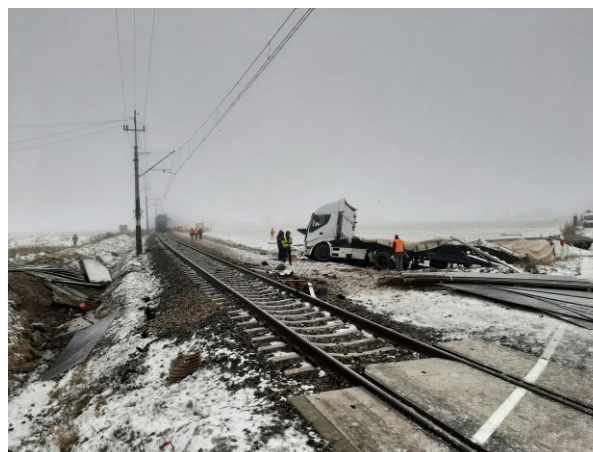
Photograph 3 - Consequences of the occurrence - the damaged lorry with semi-trailer, scattered cargo - 10 mm thick metal sheets (source: own material of PKBWK)
