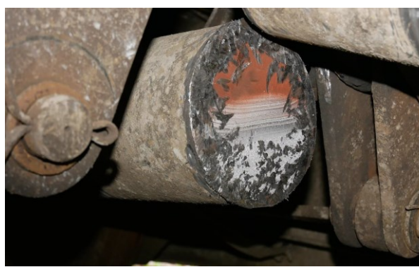
Photograph 7 - Consequences of the occurrence - a view of the fractured axle (source: own material of PKBWK)
