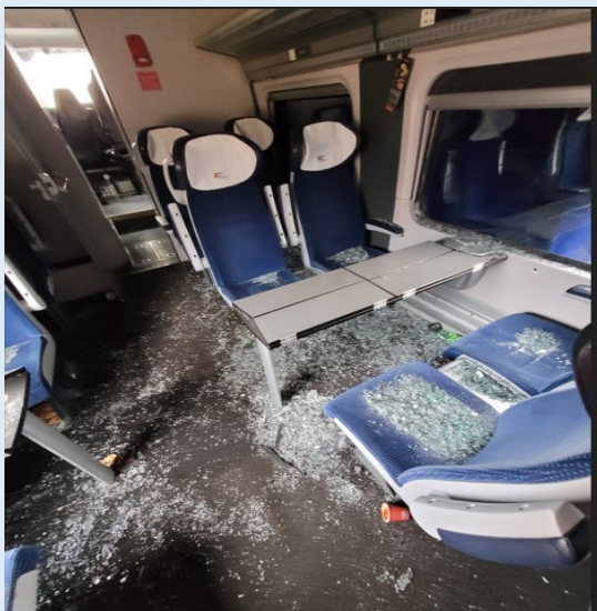
Photograph 17 - Consequences of the occurrence - the interior of ED161-004a (source: own material of PKBWK)
