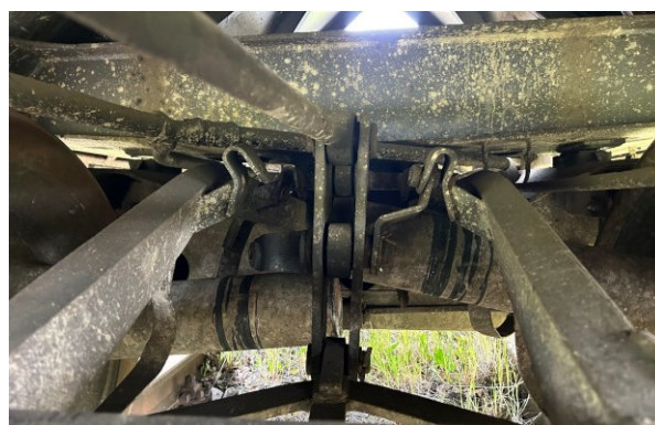
Photograph 7 - Consequences of the occurrence - a view of the fractured axle (source: own material of PKBWK)
