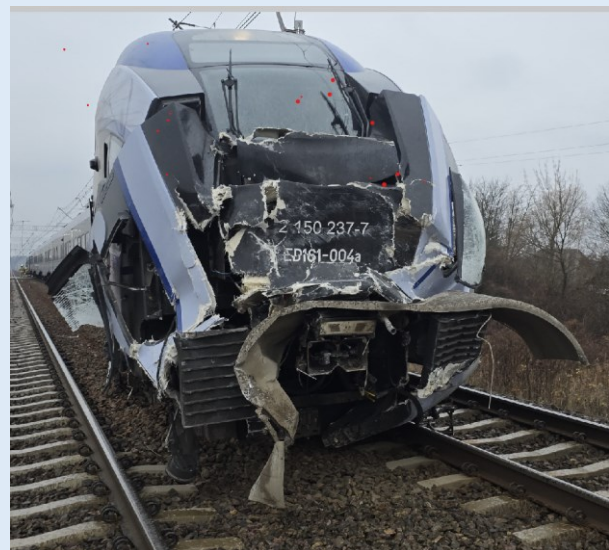
Photograph 18 - Consequences of the occurrence - the damaged ED161-004a cab (source: materials of the railway commission)
