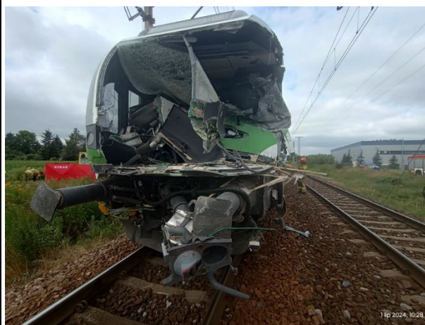
Photograph 11 - Consequences of the occurrence - a view of the destroyed driver's cab of rail vehicle ER75-001 (source: material provided by KM)
