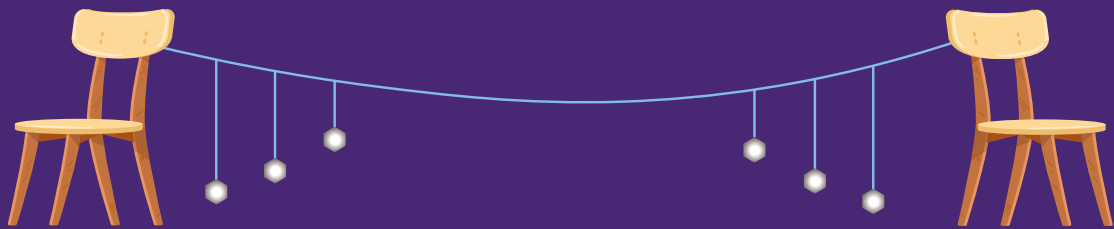
Fig. 12. Experiment with pendulums. Mechanical resonance.
