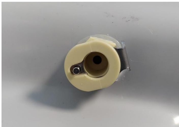
Figure 1: Leak test socket in the bowl
