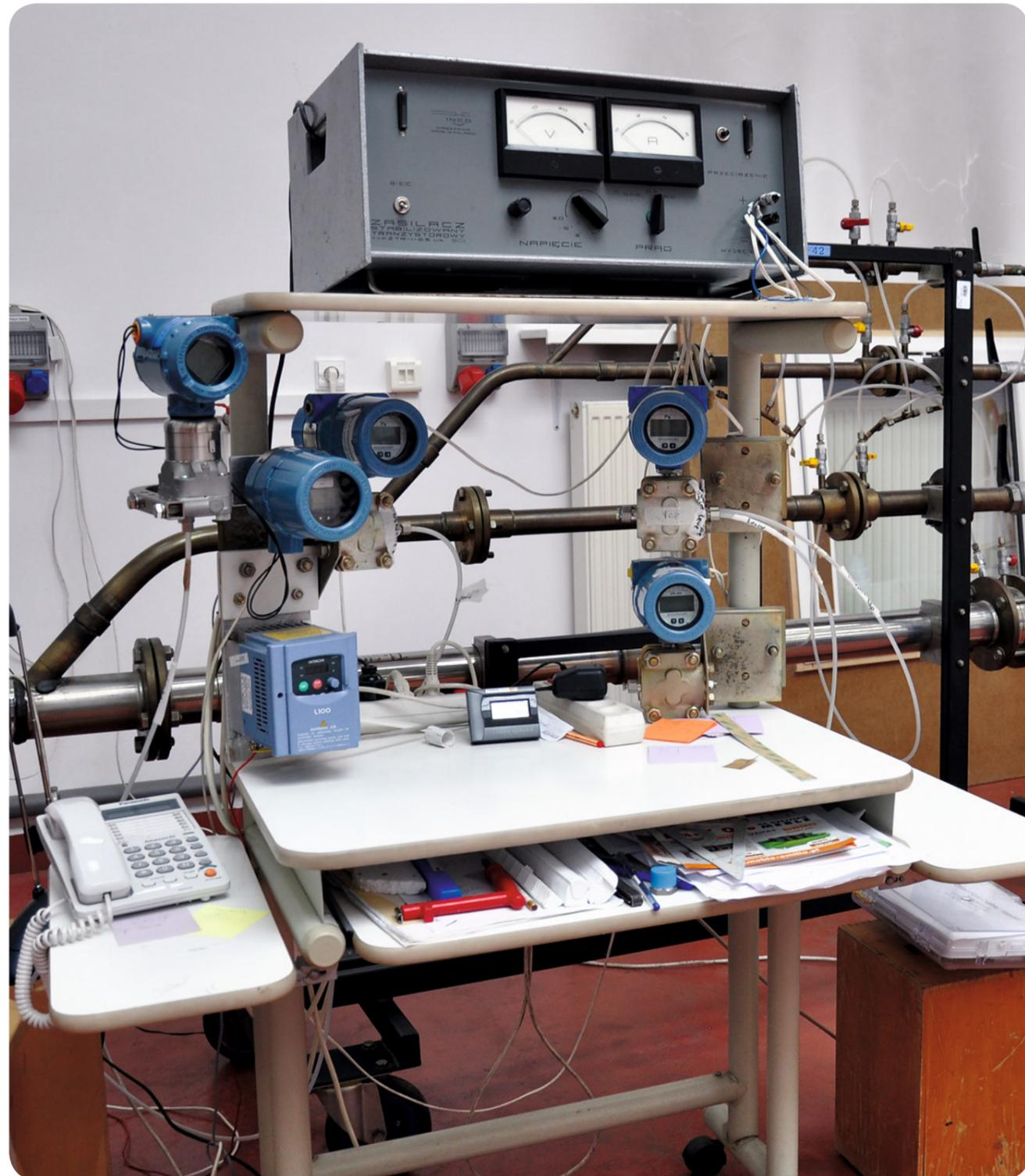
Workstation for testing flow in ventilation installations.
