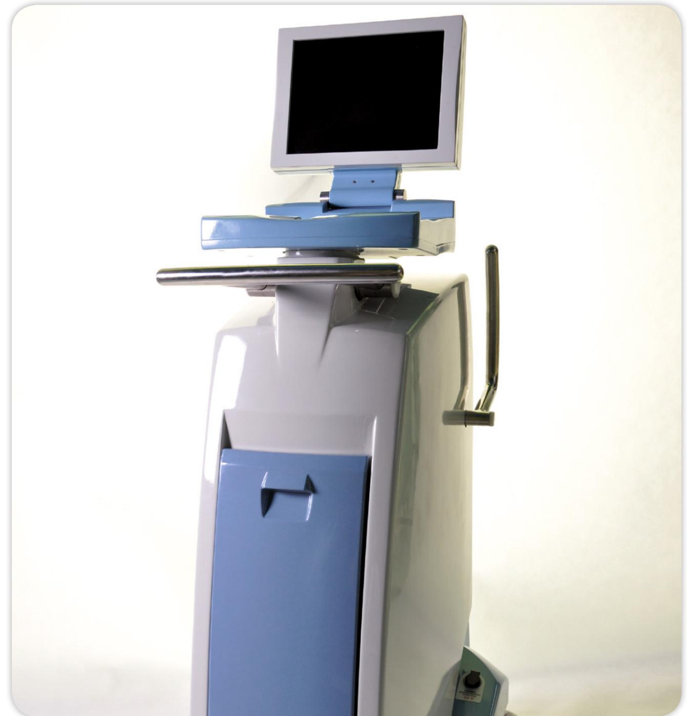
*A prototype of a mobile control panel for pulsatile blood pumps Religa Heart PDU 402.*
