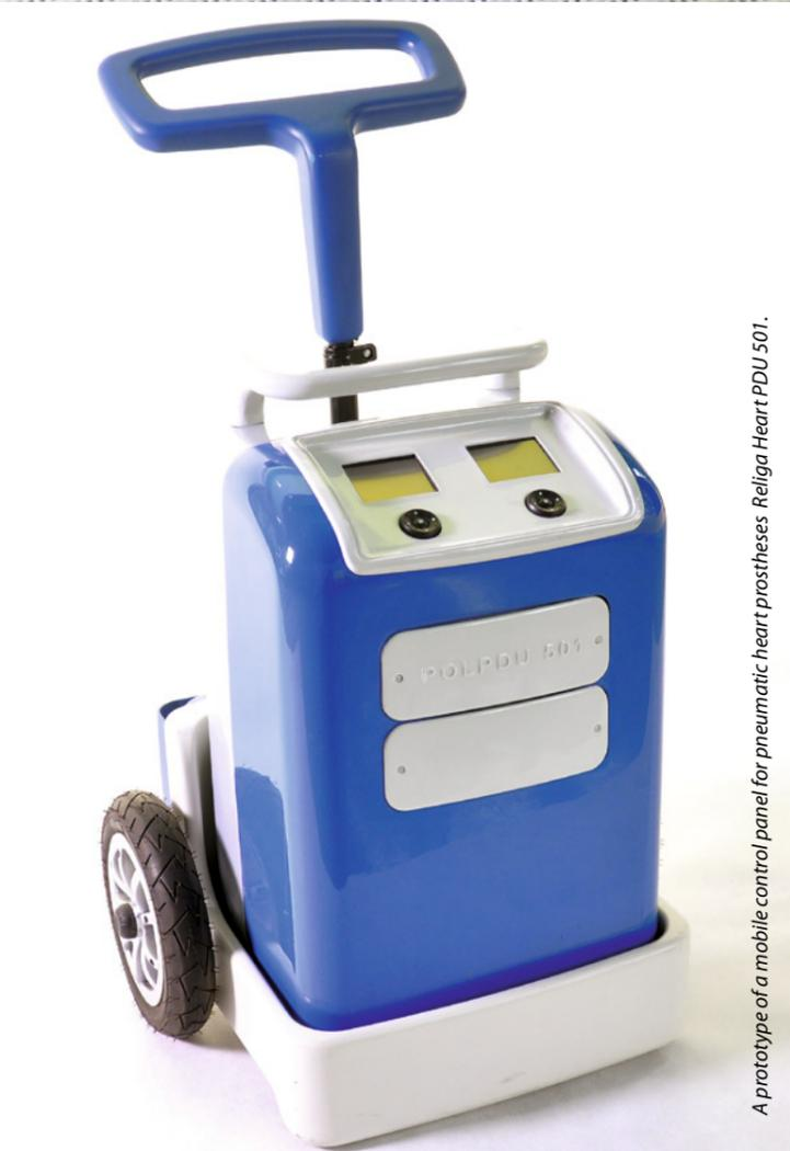
A prototype of a mobile control panel for pneumatic heart prostheses Religa Heart PDU 501.
