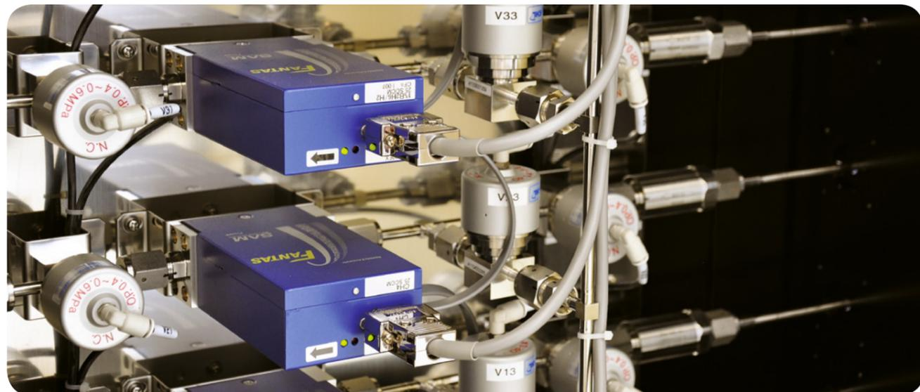
Mass flowmeters for precise metering of gases to a technological plasma chamber.
