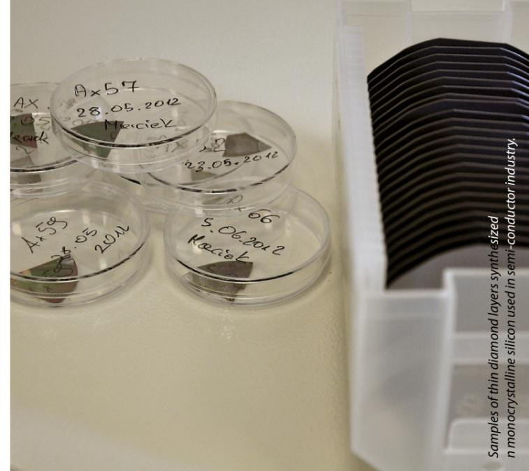
Samples of thin diamond layers synthesized on monocrystalline silicon used in semi-conductor industry.
