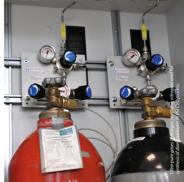
Ultra-pure gases (hydrogen, methane, nitrogen) used for synthesis of diamond layers in the CVD process.
