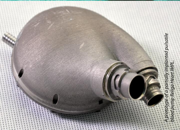
A prototype of a partially implanted pulsatile blood pump Religa Heart IMPL.
