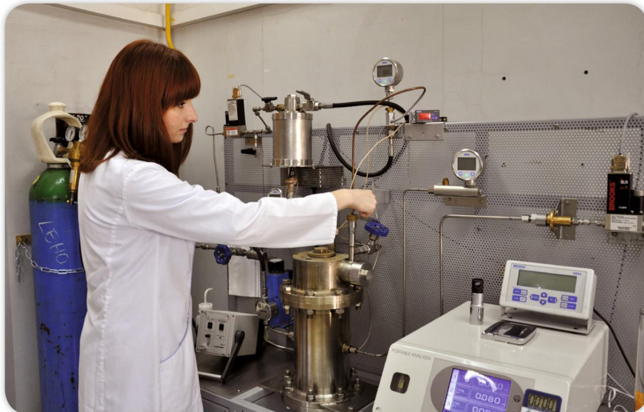
Laboratory installation for coal gasification and pyrolysis.
