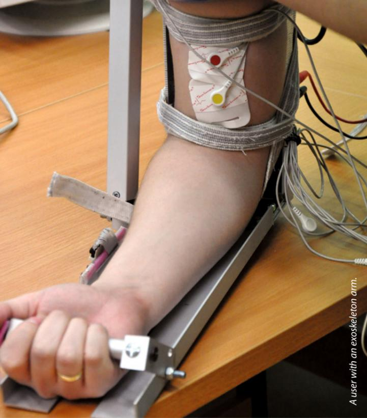
A user with an exoskeleton arm.
