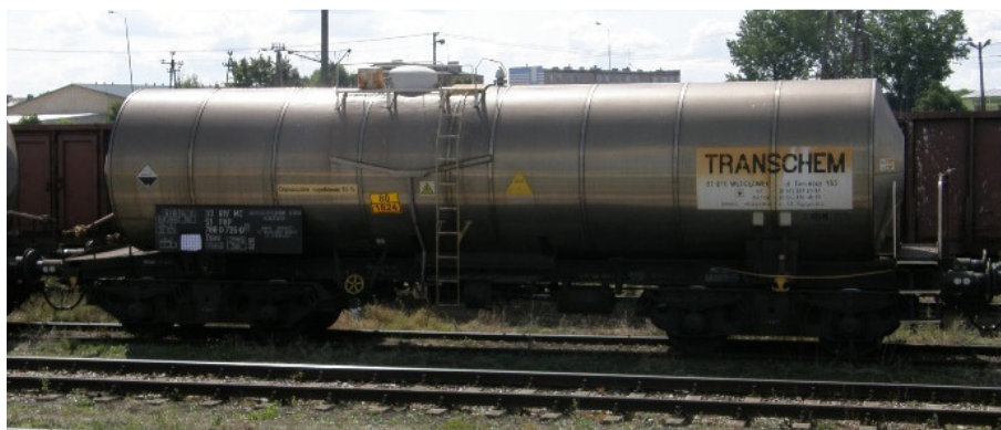
Rys. 2-142 Wagon cysterna Zaes (Transchem/PL)
