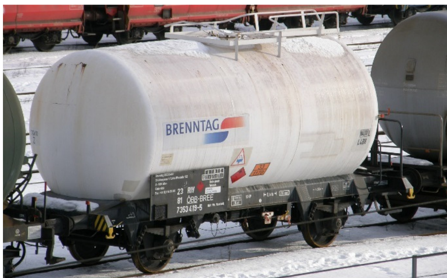
Rys. 2-127 Wagon cysterna Zs (Brenntag/AT)
