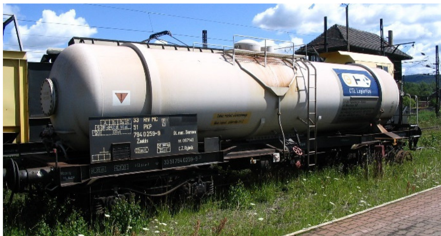
Rys. 2-143 Wagon cysterna Zaeaks (CTL Logistics/PL)
