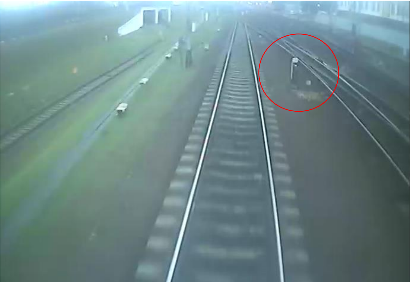
Photo 6 – View from the railbus of the shunt signal Tm30 displaying the Ms1 aspect (source: POLREGIO S.A.)
