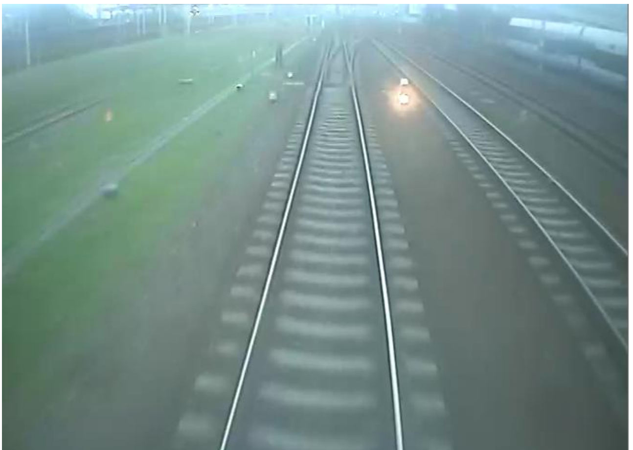
Photo 5 – View from the railbus of the shunt signal Tm37 displaying the Ms2 aspect (source: POLREGIO S.A.)
