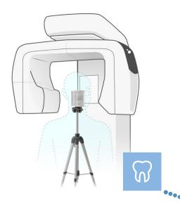
**Scan the benchmark test object** (phantom) as you would scan a patient. We provide combined "many-in-one", easy to use, universal tools for each modality, designed in a way that makes it easy to position them and perform most, if not all, tests at a single exposure / scan.
