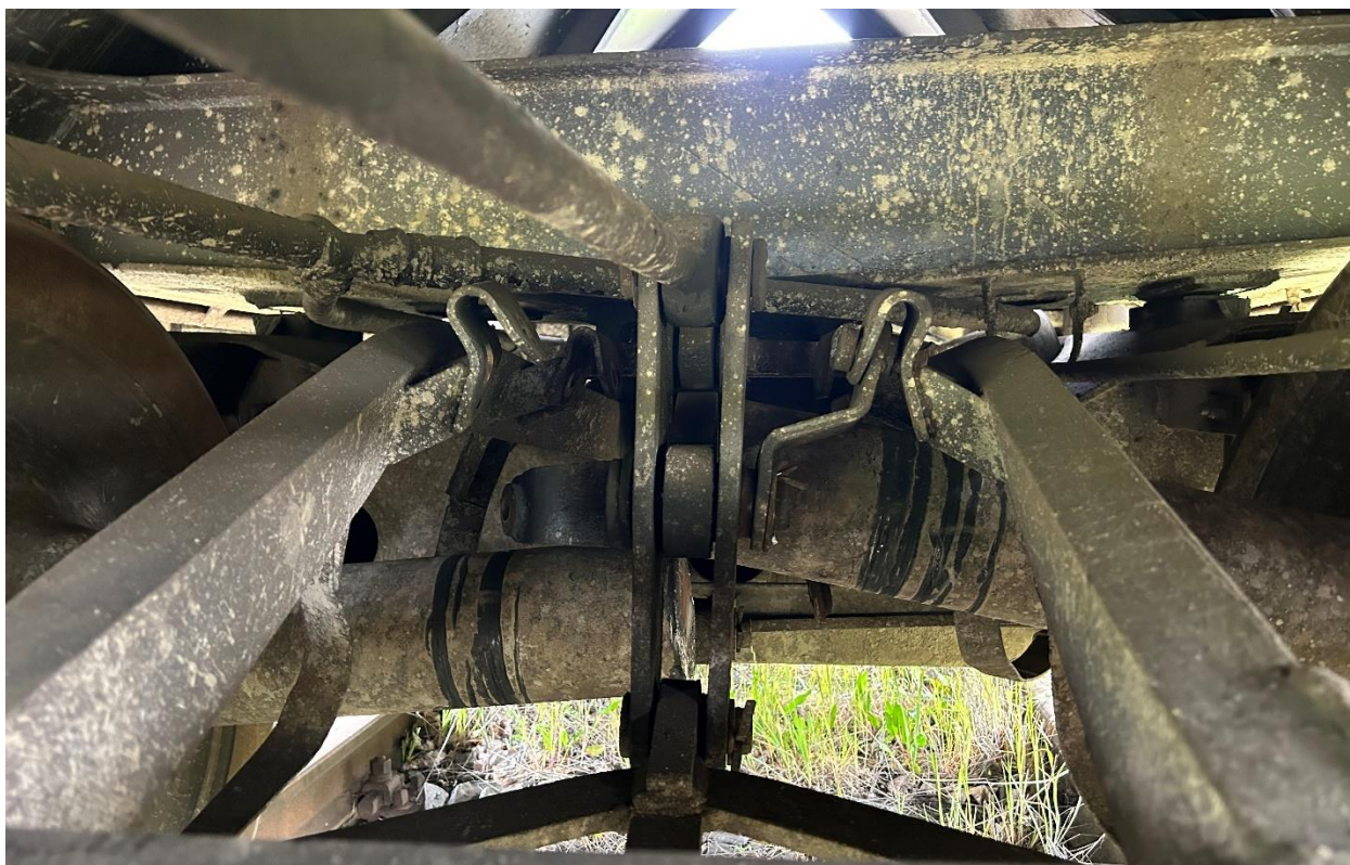
Photograph 3 - A view of the fractured axle (source: PKBWK's own material)
