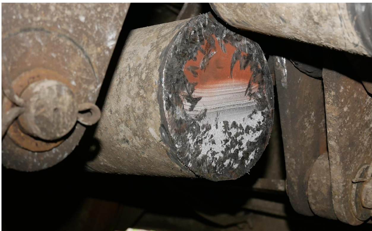
Photograph 4 - A view of the fractured axle (source: PKBWK's own material)
