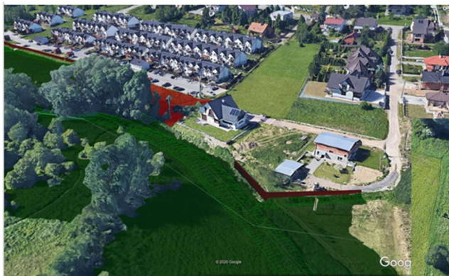
Wall in the form of a wall with a cap 44 m long and 50-70 cm high as protection against slope erosion
