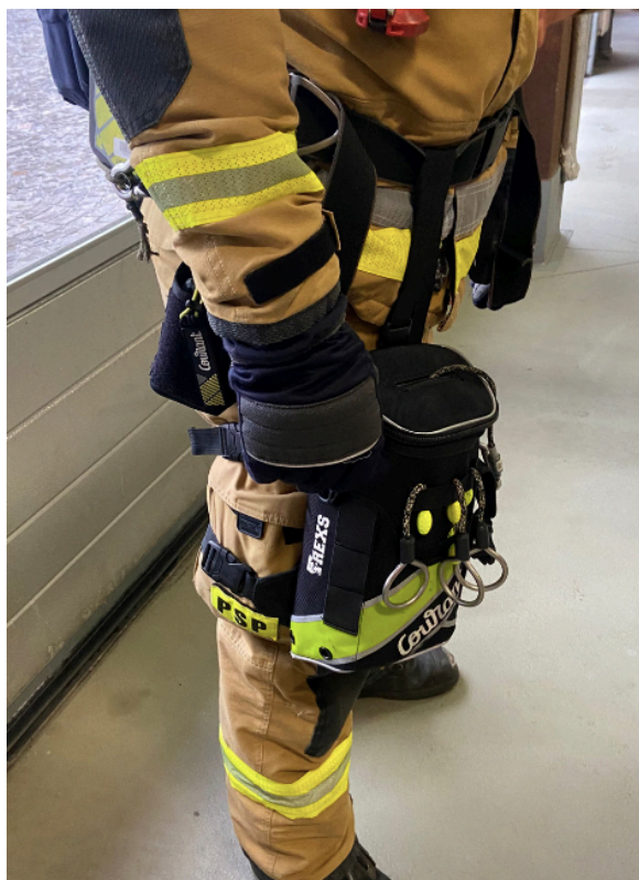
Photo: Example of a rope bag attached to a firefighter's leg. One strap is secured to the hip belt, with two additional straps fastened around the leg.
