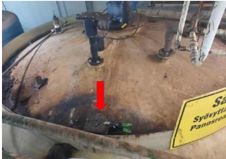
Figure 1. Sampling area of toxic gas release on the top of the waste treatment reactor
