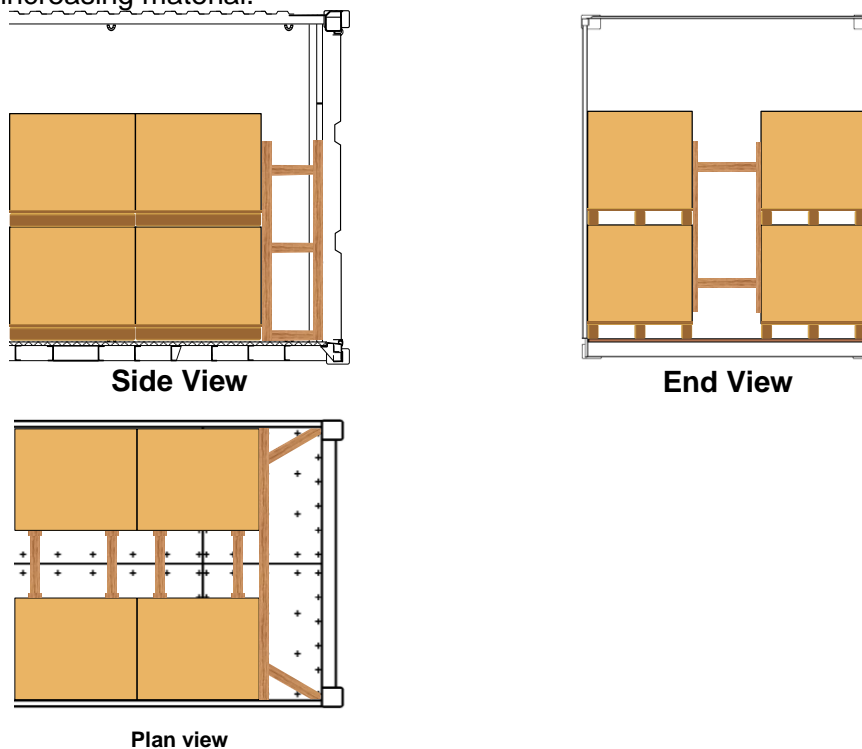
Figure 7.32 Blocking in a strong boundary CTU
