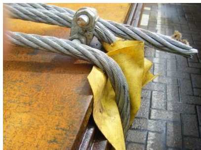
Figure 7.11 Poor edge protection
