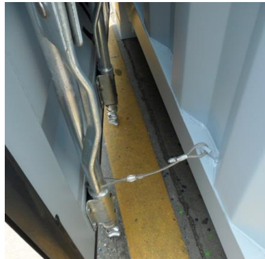
Figure 5.30 Door retaining strap
