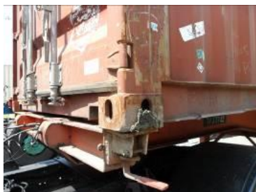
Figure 6.2 Mud in corner fitting
