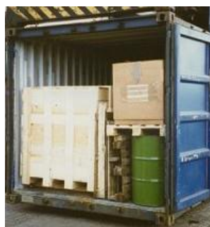
Figure 7.28 Mixed stow, use of pallets
