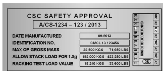
Figure 8.1 CSC safety approval plate with next examination date
