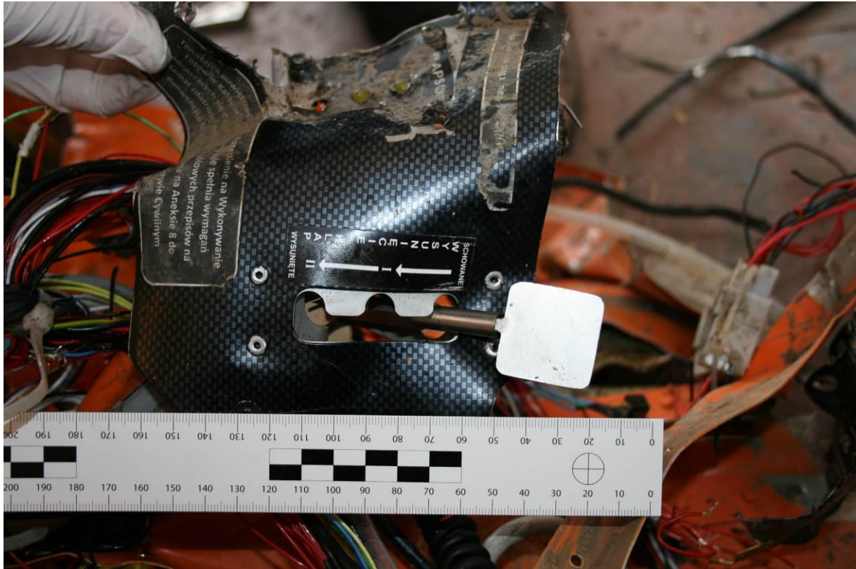
Image39 Lever for flaps extraction
