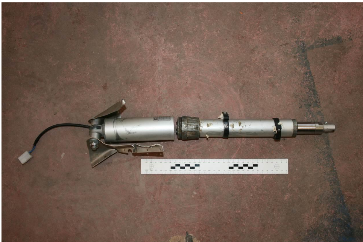
Image 40 Actuator for flaps activation
