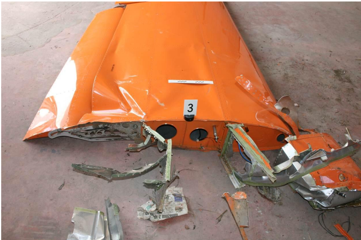
Image 38 Deformations on the left wing and wing span
