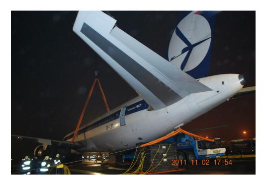
Photo 10. SP-LPC airplane plane lifted up by crane and airbags.
