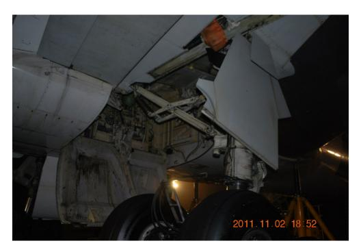
Photo 11. Extended right main landing gear after lifting SP-LPC airplane.
