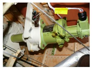
Photo 18. Electric motor of alternate landing gear extension system.
