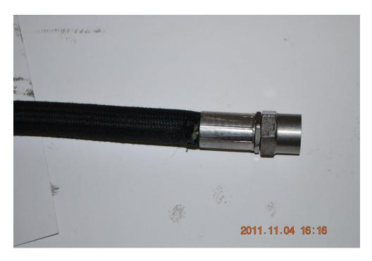
Photo14. Damage to the hydraulic hose of the landing gear extension system of SP-LPC airplane.
