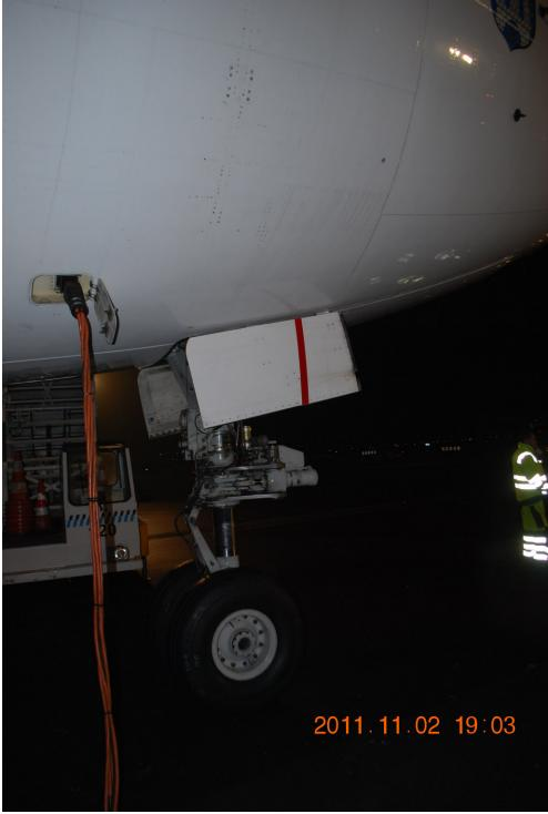
Photo 12. Extended nose landing gear of SP-LPC airplane.
