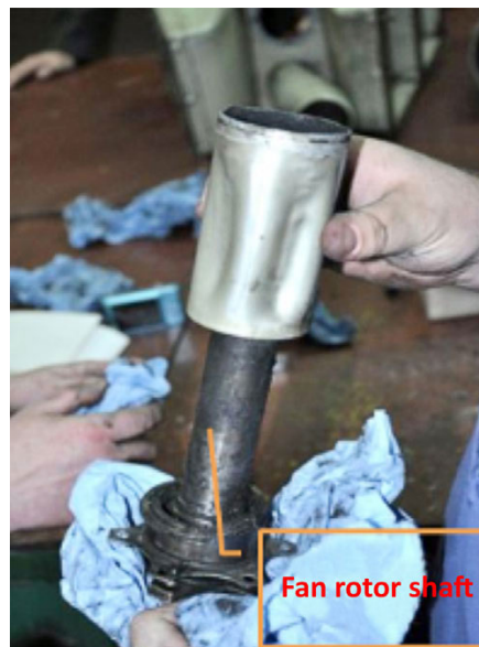
Figure 4. Dents in the outer case
