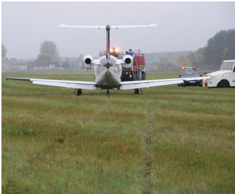
Photo 1. Landing roll traces and Embraer EMB-500 airplane after completing the landing roll.
